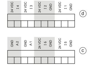
INPUTS AND OUTPUTS ARE USED ACCORDING TO PRODUCT REQUIREMENTS. MAX. LOAD FOR ALL INPUTS AND OUTPUTS I TOTAL = 300 MA CUMULATIVE !
